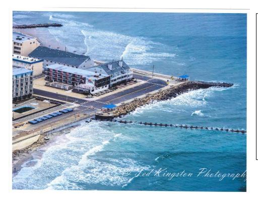
Figure 3. View taken by Ted Kingston January 2018, showing the severe depletion of the sand supply surrounding the northeast corner of the City of North Wildwood. While it is high tide in the view, the loss of beach width is serious and will require both natural and manmade assistance to correct.
