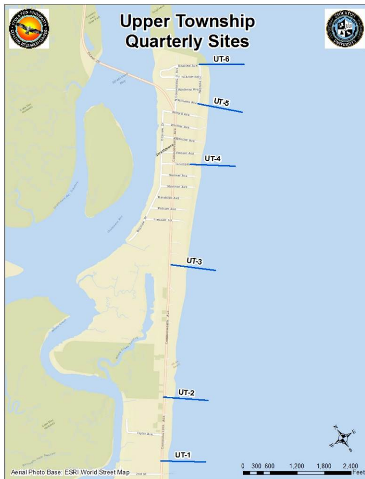
Figure 1. Locations of the 6 beach profile stations for the engineered beach in Upper Township.
