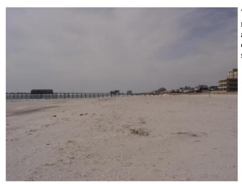
The Dorset Avenue site was also nourished during 2003/04. There was a new dune built and vegetated. The April 11<sup>th</sup> 2007 view shows the beach at the berm with the fishing pier in the distance. The dune was reestablished seaward of the original feature which was positioned just seaward of the boardwalk.
