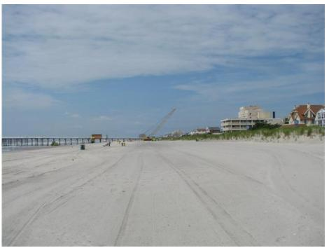
By June 27<sup>th</sup> 2008 the beach showed the presence of a berm and the dune vegetation has commenced a new growth season. The beach width narrowed by 37 feet as 16.76 yds<sup>3</sup>/ft. in sand volume moved south. This section of the Absecon Island shoreline appears to be stable since the ACOE project was completed.
