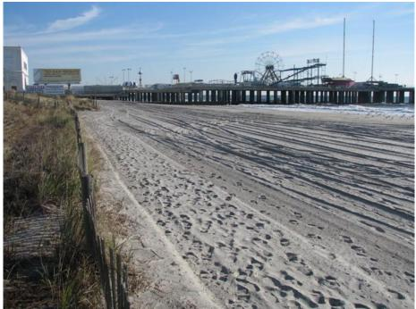
By November 26<sup>th</sup> 2008 the dune position was the same because no storm events reached the dune toe. The beach was 38 feet narrower as 35.71 yds<sup>3</sup>/ft. in sand volume moved further south. Continued erosion north of the pier has created potential for storm damage to the boardwalk should a severe storm occur.
