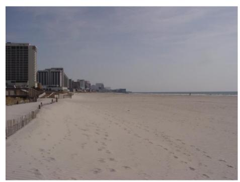
The Raleigh Avenue site received beach material in 2002 and the dune was re-configured wider and higher. On April 7<sup>th</sup> 2007 the dune had accumulated sand along a 4-foot fence established earlier. The vegetation was absent on this new foredune. The beach width still reflects the 2003-04 ACOE project as sand lost to the south has been compensated by sand moving into this area from further north.
