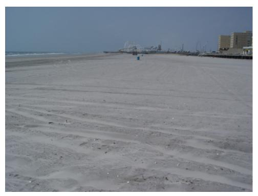
Figure 284. The photograph to the right was taken November 16, 2007 and shows the broad, flat beach leading to the recreational piers in both North Wildwood and Wildwood. This 18-month interval saw a 20.93 yds<sup>3</sup>/ft. gain in sand volume with a 54-foot shoreline advance. This annual gain is about 5% of the sand loss documented at this location.
