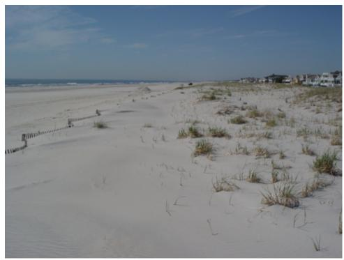
Figure 244. This view taken October 31, 2007, shows the dune between the development and the beach. This area is twice as wide as it was prior to beach restoration and provides a great measure of storm protection in spite of owner complaints that the distance is too great and the view of the ocean has been diminished. The shoreline has advanced 13 feet and the beach/dune system gained  $23.75 \text{ yds}^3/\text{ft}$ .
