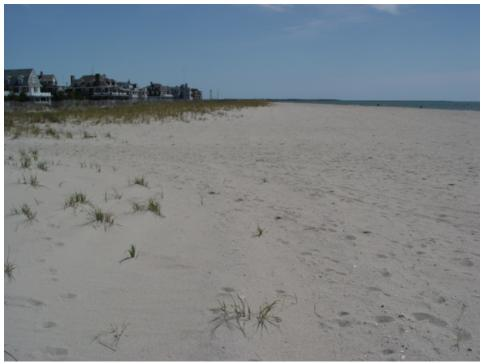
Figure 299. This view taken September 18, 2007, shows the substantial dunes between the rock revetment and the berm. 20 years ago this photo spot would have been in 5 feet of water or more at low tide. This beach gained  $8.55 \text{ yds}^3/\text{ft.}$ , and the shoreline advanced 7 feet over the study interval.
