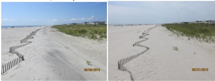
The comparison photos to the south (left taken September 5, 2014 and right photo taken August 31, 2015) show minimal changes to the dune vegetation with respect to the location of the dune fencing. This profile is located nearly in the center of the island and continued modest volumetric gains for both 2014 and 2015.
