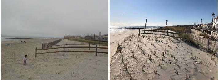
The left photo (taken October 8, 2018) shows sand placed up to the scarped dune vegetation line. The right photo (taken November 11, 2019) displays the magnitude of erosion at this location. A significant scarp has formed deep into the primary dune while the beach face has experienced continuous erosion.
