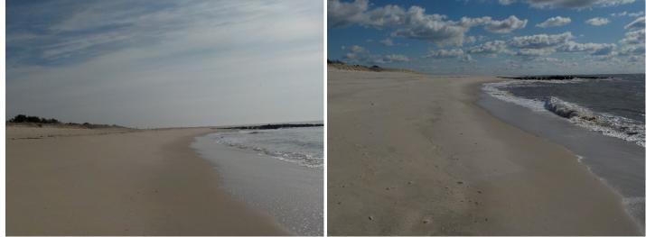
The left photo was taken on November 19, 2018. The right photo was taken on November 8, 2019. Sand was added by the USACE as far west as this groin cell in Cape May Point by spring 2017 with loss in beach width through May 2019. However, by the fall 2019 survey, the beach width reversed this trend, and expanded seaward.
