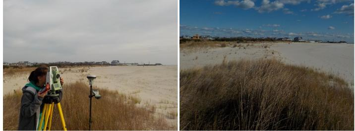
The left photo was taken November 19, 2018. The right photo taken on November 8, 2019, and shows a narrower beach 18 months later. The dune system remained very stable but changes in the beach elevations and berm positions have taken place throughout the four surveys conducted.
