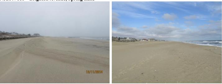
By December 11, 2014 (left) the USACE had added 40.47 yds<sup>3</sup>/ft. in new sand advancing the shoreline by 13 feet. The right view on November 29, 2015 shows the wide beach with an active surf zone breaking on an offshore bar.
