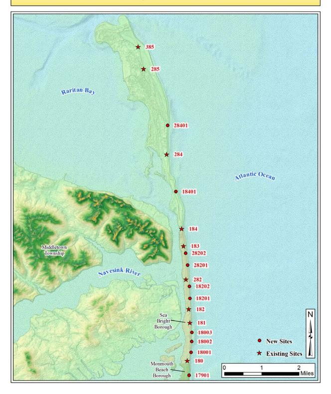
Figure 1b. Reach 2 showing Sandy Hook and Sea Bright survey site locations. The USACE NY District sites added in the fall of 2017 have 5 digits as location numbers. Site #385 was added spring 2017 to extend the Sandy Hook oceanfront beach coverage closer to the tip of the spit to gain better information on sand volumes moving north from the federal project.
