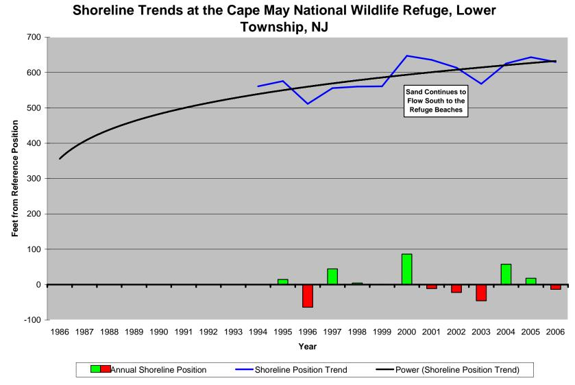
**Figure 186.** Site 208. Established within the natural area of the Cape May National Wildlife Refuge in 1994, this site shows the impact of the 1911-vintage Cold Springs Inlet jetties in trapping sand. The area has been constructional for decades.
