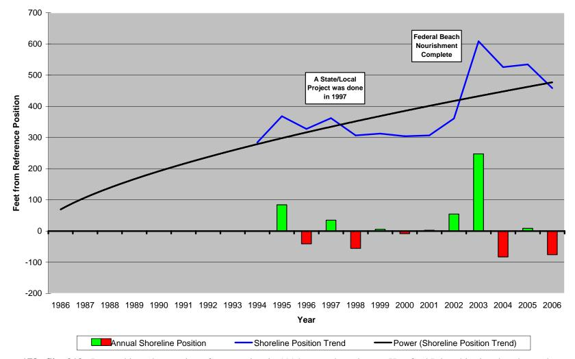
**Figure 178.** Site 212. Inserted into the rotation of survey sites in 1994 to get data close to Hereford Inlet, this site also shows the impact of the Federal project completed in 2003. Similar losses at this location have cut back the total volume as the shoreline
