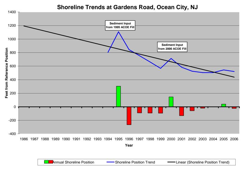
**Figure 148** – **Site 225.** This site was established in 1994 to provide information near Great Egg Inlet. This profile line is strongly influenced by sand placement events on the oceanfront beach. During the years following the sand placement, the beach expanded as
