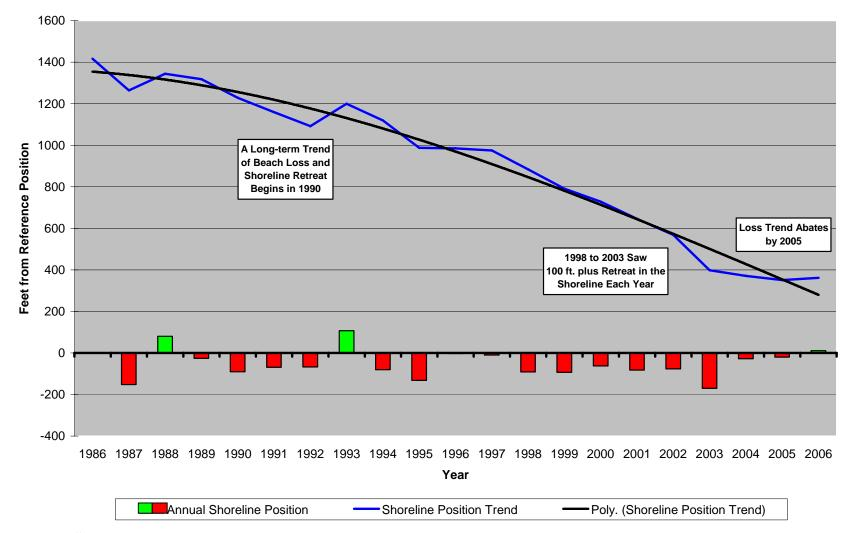
**Figure 180. Site 111.** North Wildwood takes the prize as the most erosional location in New Jersey, the opposite of site 245 in Barnegat Light Borough where the Barnegat Inlet jetty causes the greatest shoreline advance. The initial shoreline position was
