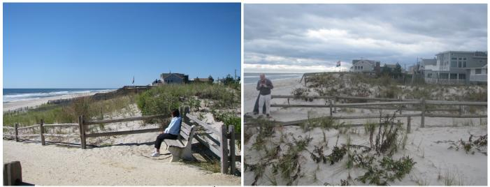
The photographs above were taken on September 11<sup>th</sup>, 2012 (left) and November 1<sup>st</sup>, 2012 (right). Both images show the view of 20<sup>th</sup> Street (site 241) looking south. This location in Surf City received a beach replenishment in 2007, which increased the sand volume and width of the dune and berm. The dune and berm both experienced substantial erosion; however no overwash occurred at this location.
