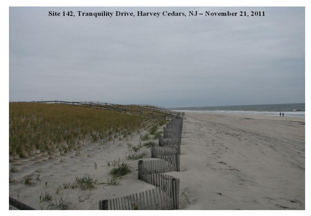
Figure 222. Shown above is the view looking north from the fence line at Tranquility Drive in Harvey Cedars, NJ. The sand trapping effect of the dune fencing is apparent in this picture.
